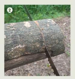
2. With the wood held securely in a sawhorse, saw a groove in the bark side about 5 or 6cm from the end. The groove should stop at least 2cm from the flat side of the wood.
