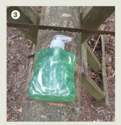
**3.** Place the bottle on the wood as shown, to measure how tall the stand needs to be. Saw it off a few cms beyond the top of the pump handle when it is extended.
