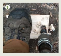
8. Turn the wood over and drill a large hole using the bit and brace. This hole should have a diameter as wide as that of the pump handle. It should be a couple of cms deep but not go all the way through the wood.
