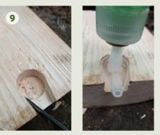
**9.** Use the knife to carve a tapered channel from the auger hole to the edge that will house the nozzle of the pump handle.
