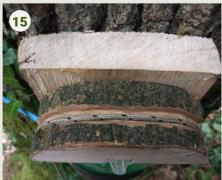
**15.** Cut a length of paracord a bit longer than twice the height of the ground to the top of the pump block. Find the middle and place it in the groove at the top of the pump block.
