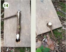
**14.** Cut a peg to hold the front of the pedal in place through the big hole.
