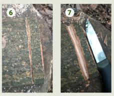
6. Time to use the offcut from cleaving to make the top block that will press on the pump handle. Saw a groove a few mm deep, all the way around the bark side. This should be about 1cm from the end of the wood. Pay attention to holding this short length of wood safely while you saw.
