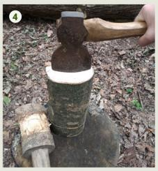
**4.** Place the wood upright on a stump and very carefully measure up where to cleave with your axe or froe. The aim is to remove the section of wood above the groove, leaving a backplate with an integrated shelf. It will look like a high backed chair.
