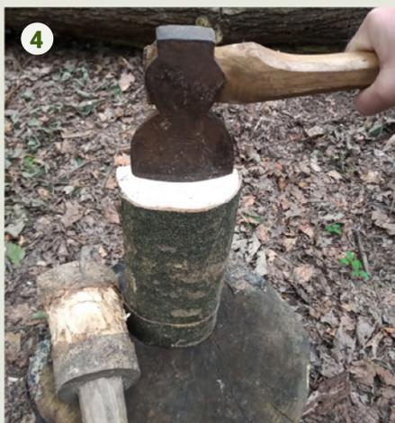
**4.** Place the wood upright on a stump and very carefully measure up where to cleave with your axe or froe. The aim is to remove the section of wood above the groove, leaving a backplate with an integrated shelf. It will look like a high backed chair.
