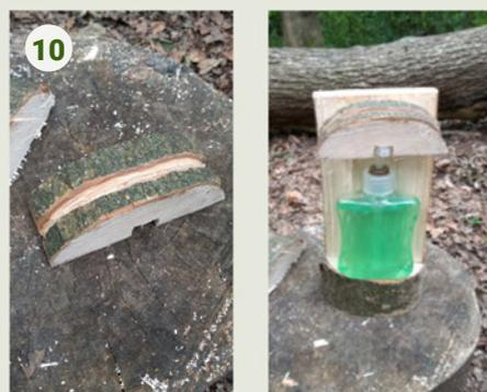
**10.** Turn the wood over and saw off the section that you have been working on. The gap from the back of the drilled hole to the back edge of the wood should be small enough to not touch the back piece of the stand when the device is assembled.
