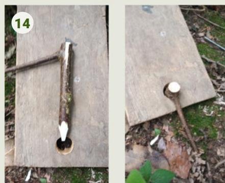
**14.** Cut a peg to hold the front of the pedal in place through the big hole.
